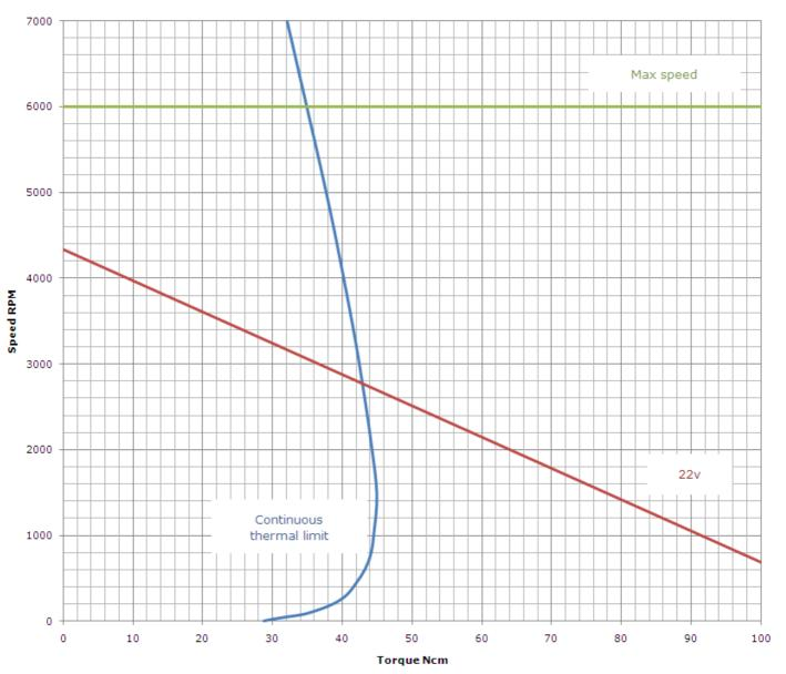
NOTE: The angle of the Torque/Speed curve remains the same for higher and lower voltages. The speed varies proportionally from zero rpm relative to the voltage supplied. The stated voltage is an example, not a predefined maximum or minimum. Due to ongoing product improvement data in this datasheet maybe subject to change without notice.
