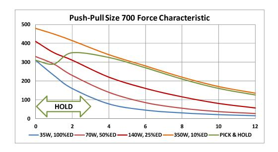
realised at the extended position similar to an intermittent duty curve, with continuing excitation power comparable to (or even lower than) that of the 100% duty curve.
