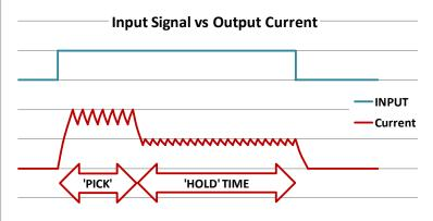
showing greater force with increasing excitation power, and the shape of the curve with force increasing as displacement reduces towards zero are similar for most linear solenoids), the use of a pick and hold circuit enables force to be realised at the extended position similar to an intermittent duty curve, with continuing excitation power comparable to (or even lower than) that of the 100% duty curve.
