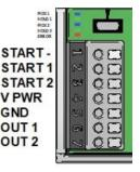
Terminals 1 (Negative), 2 (Start1) and 3 (Start2) are the opto-isolated control inputs. The input circuit is as shown below, applying 5v-30v to this will switch the circuit 'ON'. Higher control voltage may be used if appropriate serial resistor is inserted to limit the input current to 6mA.
