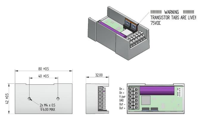
The standard module configuration is mounted in a die-cast box and potted (encapsulated) with resin.
