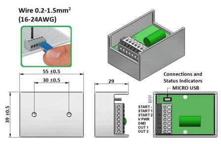
Standard module configuration is mounted in a die-cast box and potted (encapsulated) with resin.
