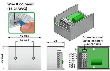
The standard module configuration is mounted in a die-cast box and potted (encapsulated) with resin.
