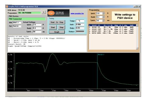
The 'Graph' display shows the current vs time for an interval of 1.5x the chosen 'Pick' time. The graphical display allows the user to visualise the following parameters:
