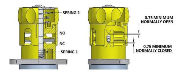
In the PV24-CO2 changeover valve, the spring configuration looks as above. The lower spring 'Spring 1' pulls down the pinch bar assembly and provides the closing force. The upper spring 'Spring 2' holds down the tube clamp to
