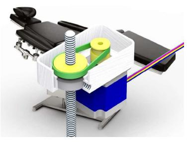
The rotating element of the actuator needs to be supported by a bearing having sufficient load capacity to support the axial load.
