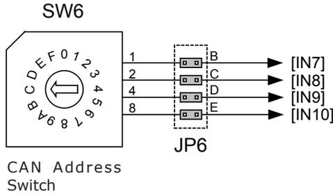
Note: To use inputs 7,8,9, or 10 as logic inputs remove jumpers shown at left to disconnect SW6 from logic inputs.
