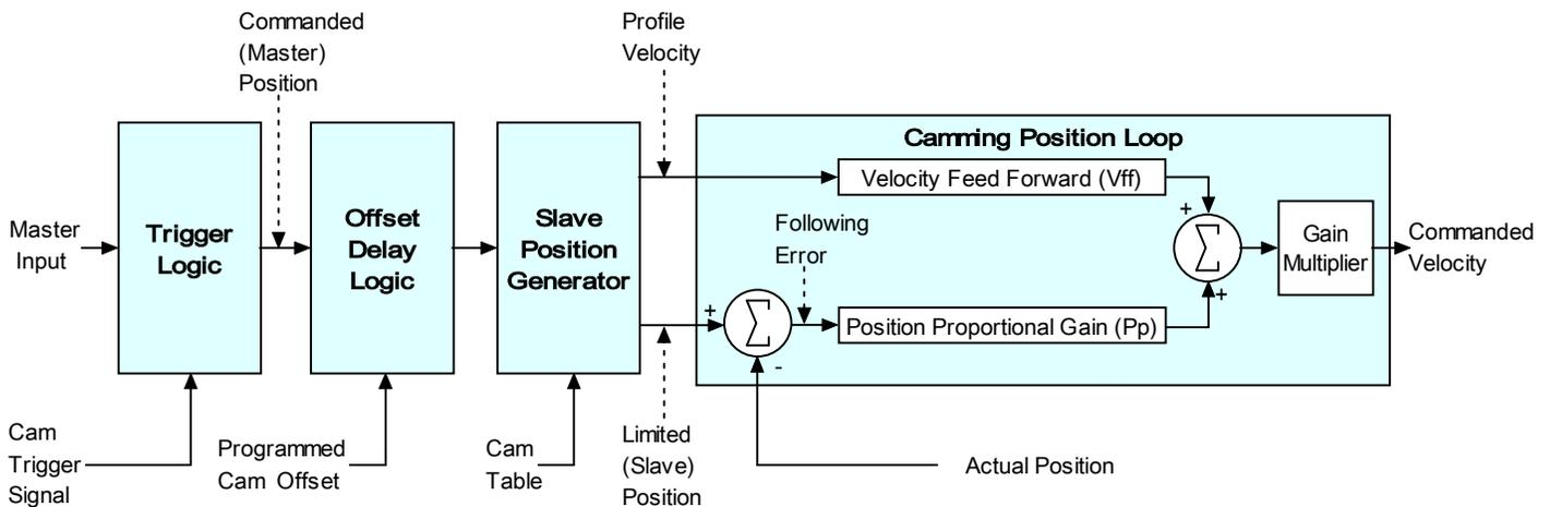
Note that during camming, profile velocity, acceleration, deceleration, and Aff have no effect. The only limiting variables are the current limits and the velocity limit in the velocity loop.
