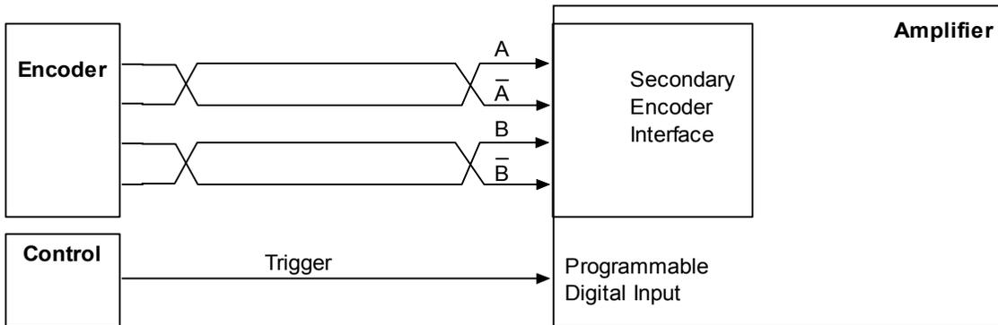
To operate correctly with this combination of connections, be sure the amplifier and camming configuration includes the following settings:
