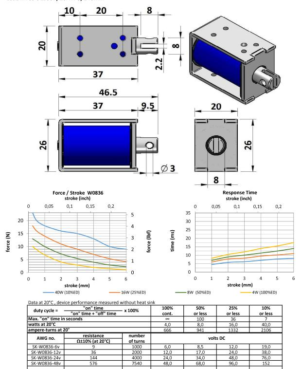
Insulation Resistance >100M $\Omega$ , 500VDC Megger
