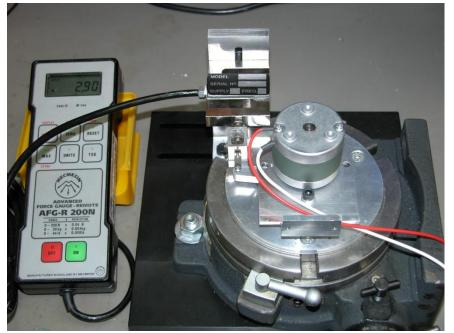
the part energised from a regulated current source. **Current regulation** stabilises the response time of the solenoid against variations in supply voltage or operating temperature. The solenoid is energised with specified current condition, and is rotated whilst monitoring torque output to derive the torque curves. The torque is measured turning in either direction, and the lower of the two measured
