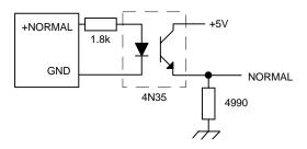
If a FAULT signal is required, then reversing the connections to the input led of the optocoupler will provide it, as shown below.
